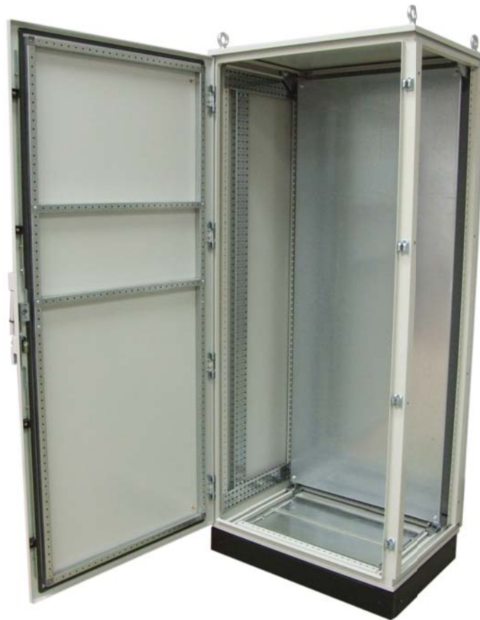
Frame surfaces feature square (for cage nut) and round holes at 25mm centers for convenient mounting (like optional light kits as shown).
