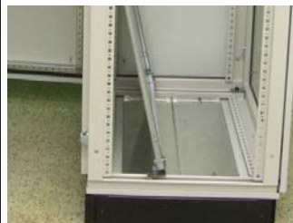
Inner panel slides easily along bottom strut channels and hooks over bottom panel supports.
